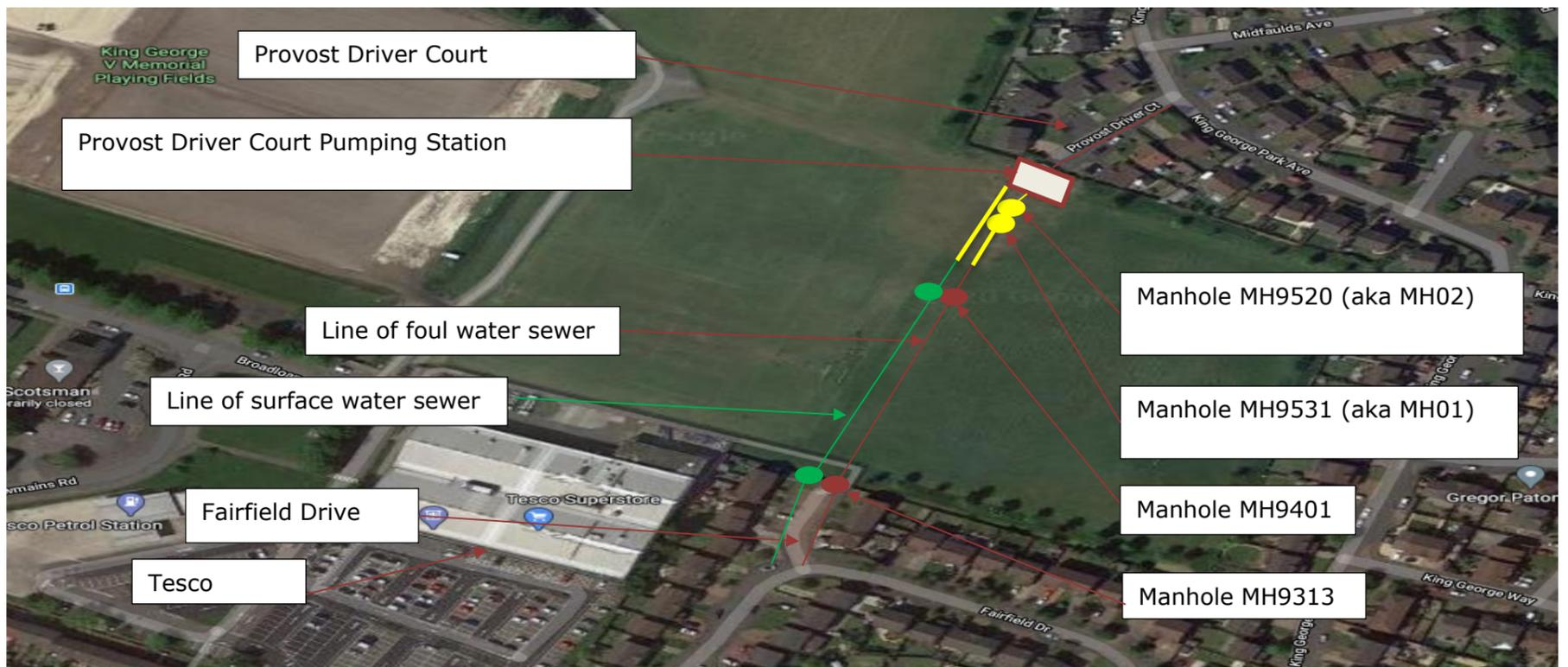
These works to repair a damaged section of waste water pipe will help return the existing pumping station to full operation, removing the need for continued Scottish Water site presence.
